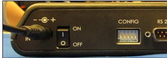
External Motion Tracker Power Switch
