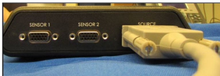
The External Motion Tracker Source Port
