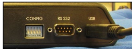
The External Motion Tracker USB Port
