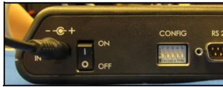
The External Motion Tracker Power Port
