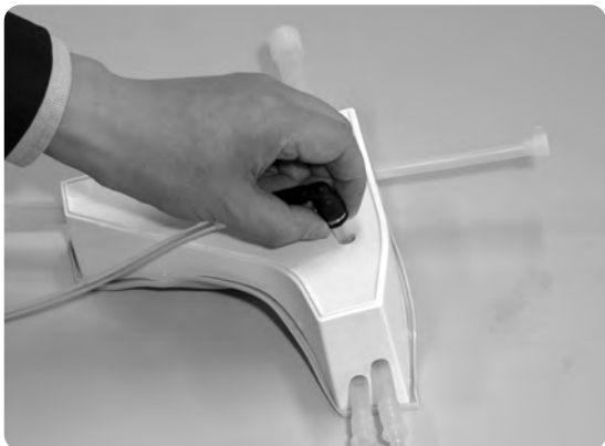
Disconnect the pulsation unit from the pad. The tube can be disconnected by pushing the stopper ring toward the connector.
